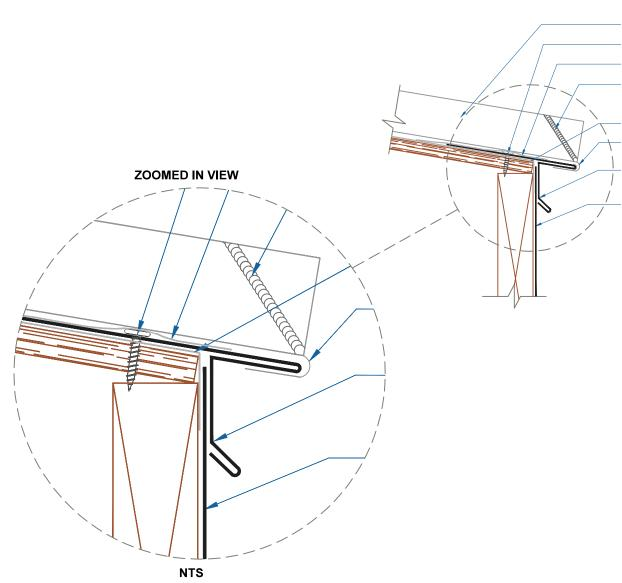
**DMC 175S PANEL** #10 - 13 x 1" PHW (12" o.c.) METSHIELD UNDERLAYMENT DREXEL APPROVED TUBE SEALANT (FIELD APPLIED BETWEEN PANEL RIBS) **METSHIELD UNDERLAYMENT** FIELD CUT & HEM PANEL 180°
