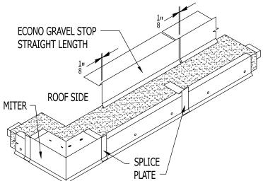
**STEP 4: Installing Econo Gravel Stop Straight Lengths**Place a Splice Plate in the opposite end of the installed Miter or End Cap.
