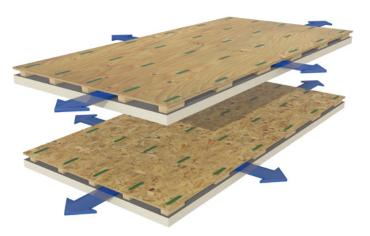
Defend-R Vent is a venting composite insulation board that consists of a 4' x 8' panel of closed cell rigid polyisocyanurate, a middle layer of solid wood spacers, creating a standard 1" air space and a top layer of APA/TECO rated OSB or plywood. Defend-R Vent is the environmentally intelligent choice for steep slope roofing applications and is viable in green and sustainable building designs.
