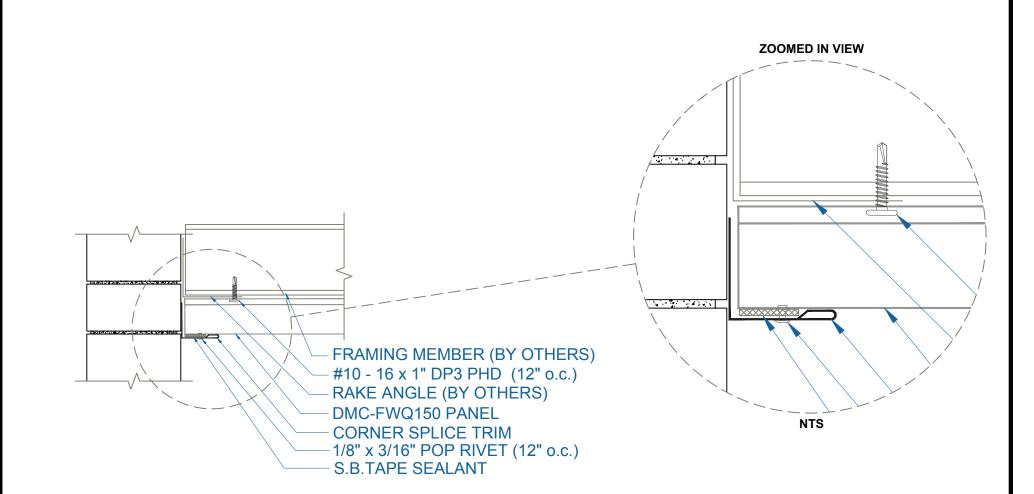
SOFFIT TO WALL SCALE: 3" = 1'-0"
