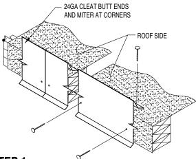
STEP 1 : Installing Secure-Lok 24GA Galvanized Cleat
