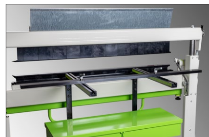
The T-groove back gauge allows flexible set-ups and great repeatability. Max. back gauge depth 585 mm. (Option)
