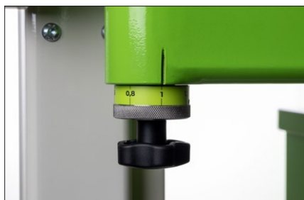
Adjust the sheet thickness on the fly to get perfect results.
